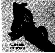
The new procedure for adjusting the Kompac form roller stripe now eliminates turning eccentrics. The set screw at the end of the bracket foot now adjusts the form stripe. Turning the set screw clockwise causes a lighter stripe. Turning the set screw counter clockwise causes a heavier stripe.
